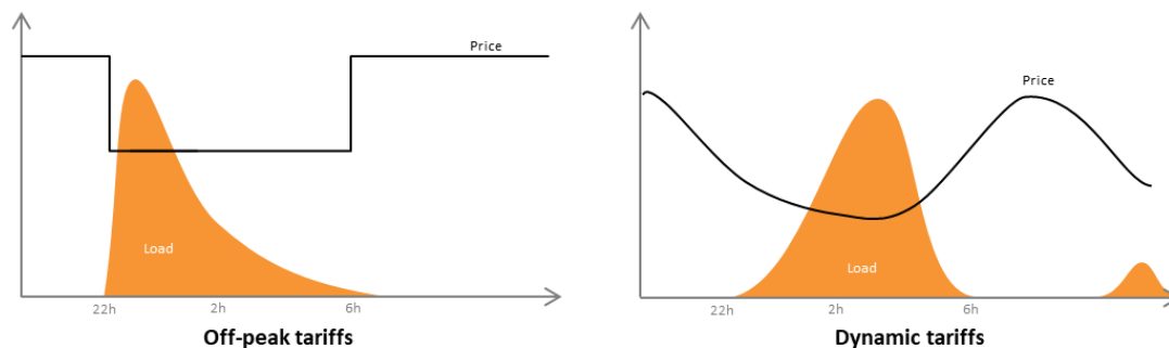
Figure 3 - Power load from a large number of EVs charging depending on tariffs
