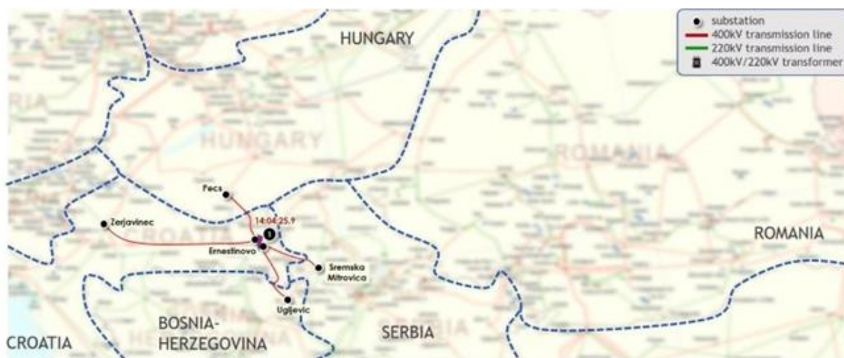
Figure 4.2.25 Power flows before the CE SA separation caused by the incident on 8 January 2021
