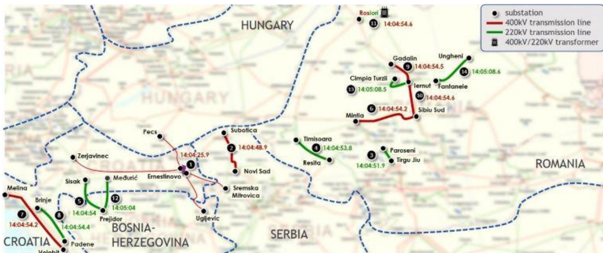
Figure 4.2.26 Transmission line outages during the incident on 8 January 2021
