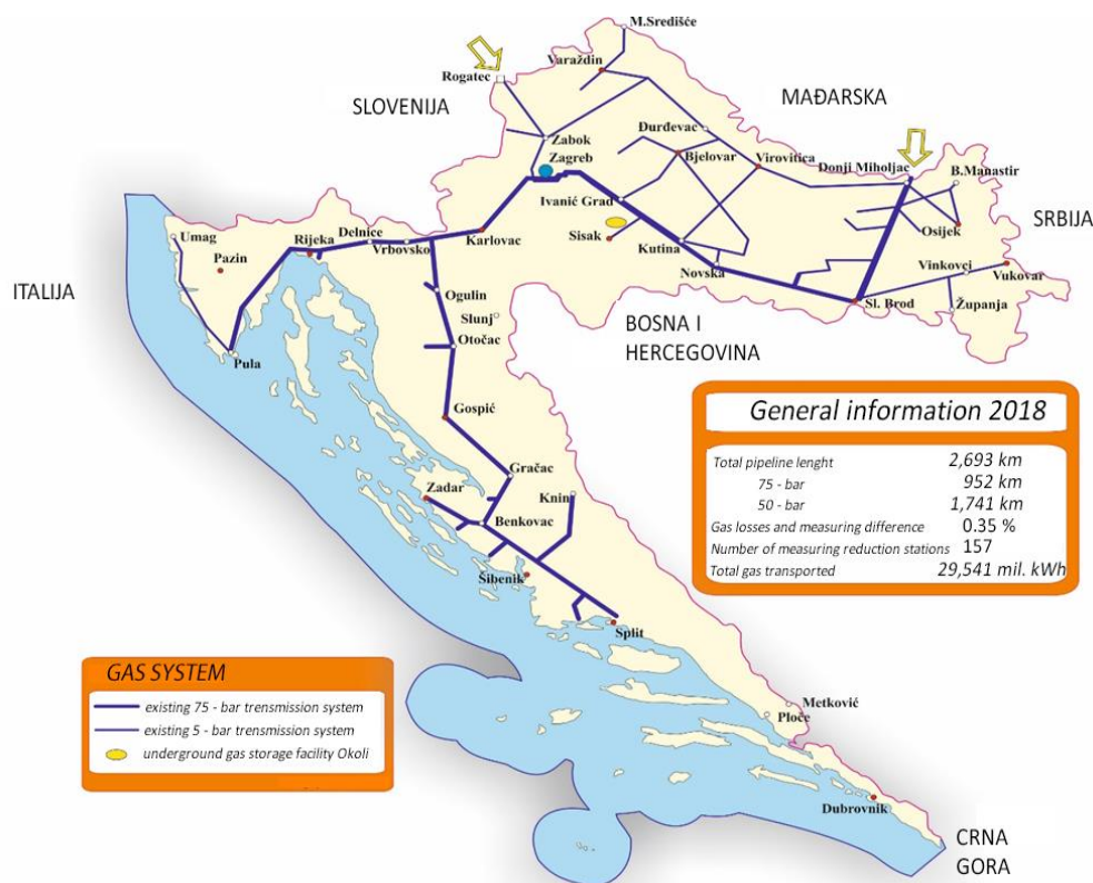
Figure 5.2.1 Croatian gas transmission system
