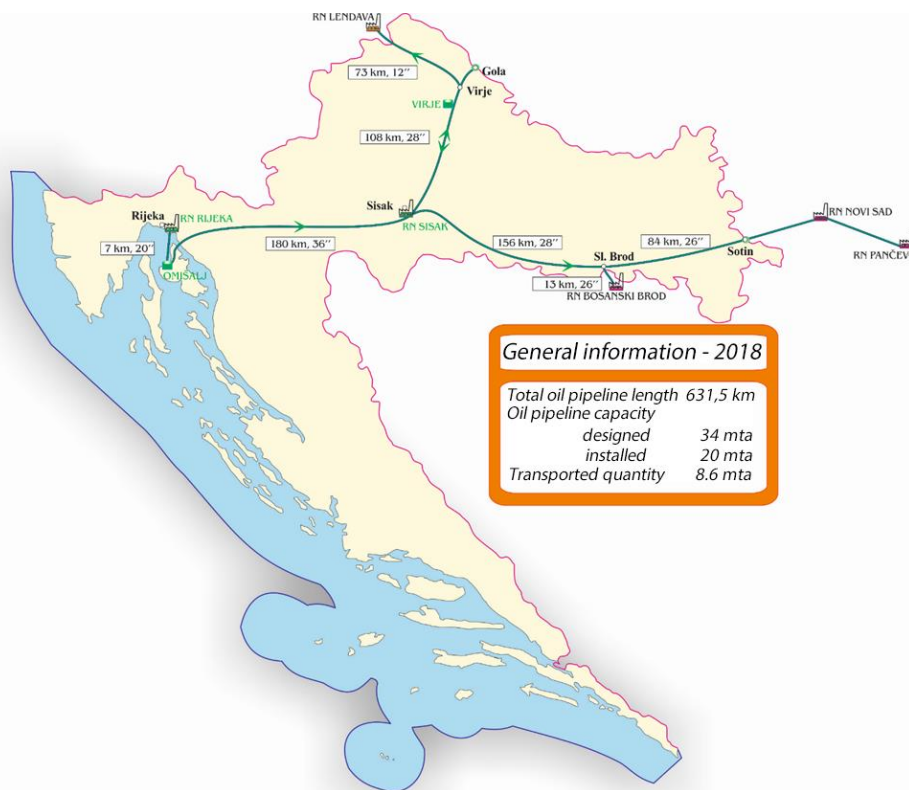
Figure 6.2.1 JANAF d.d. oil pipeline system
