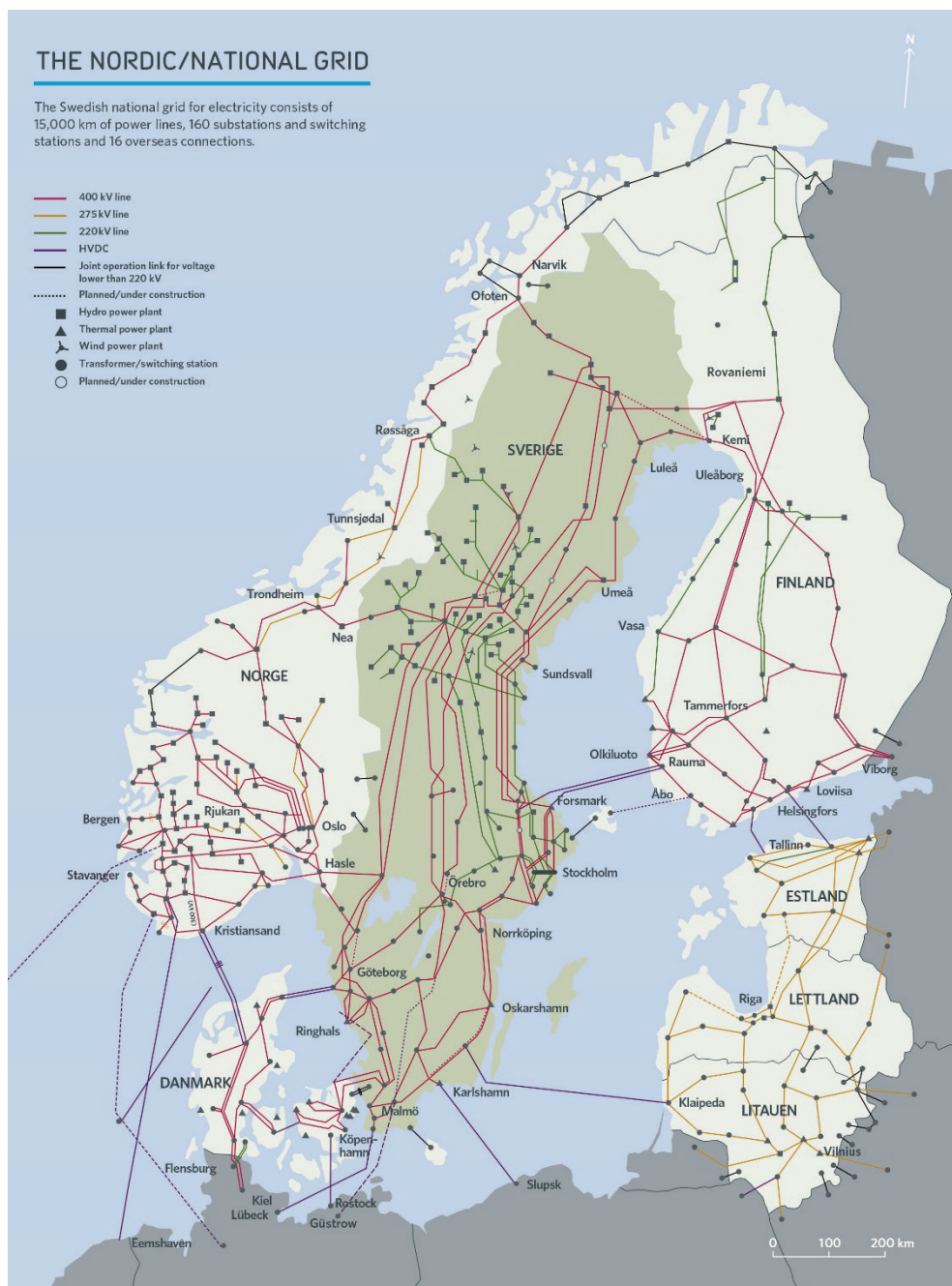
Figure 1. The Swedish transmission network for electricity and other connections to other countries
