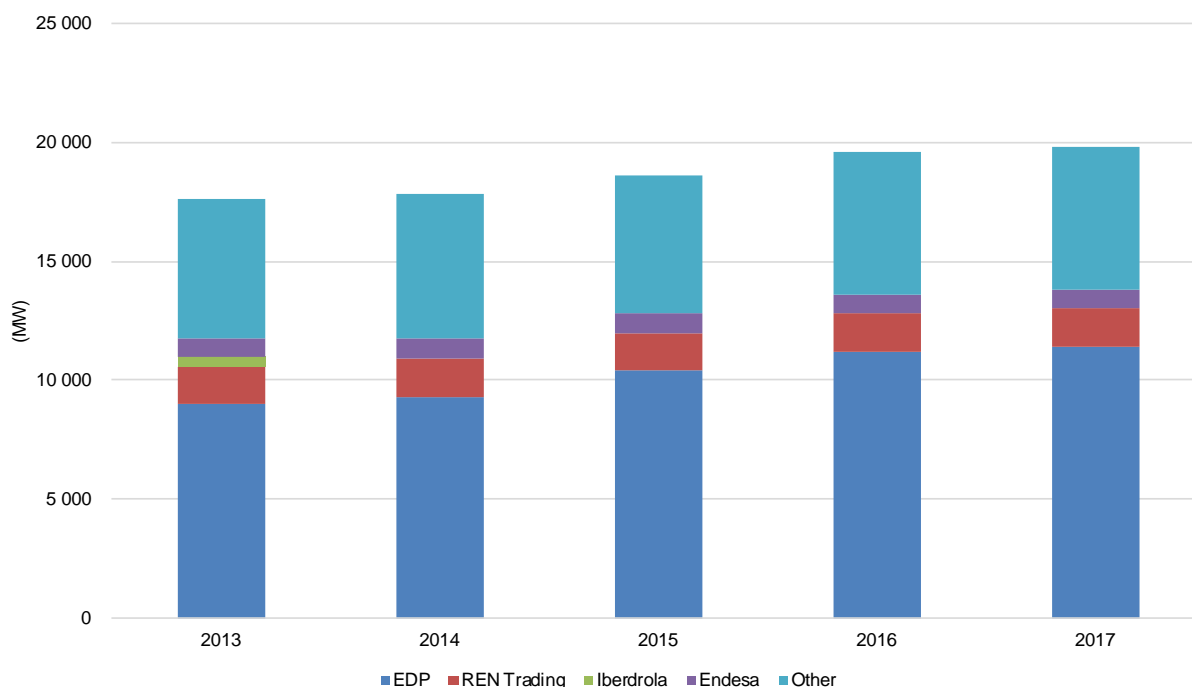
Figure 3-18 - Description of the electricity generation installed capacity in Portugal (by agent and installed capacity), 2013 to 2017
