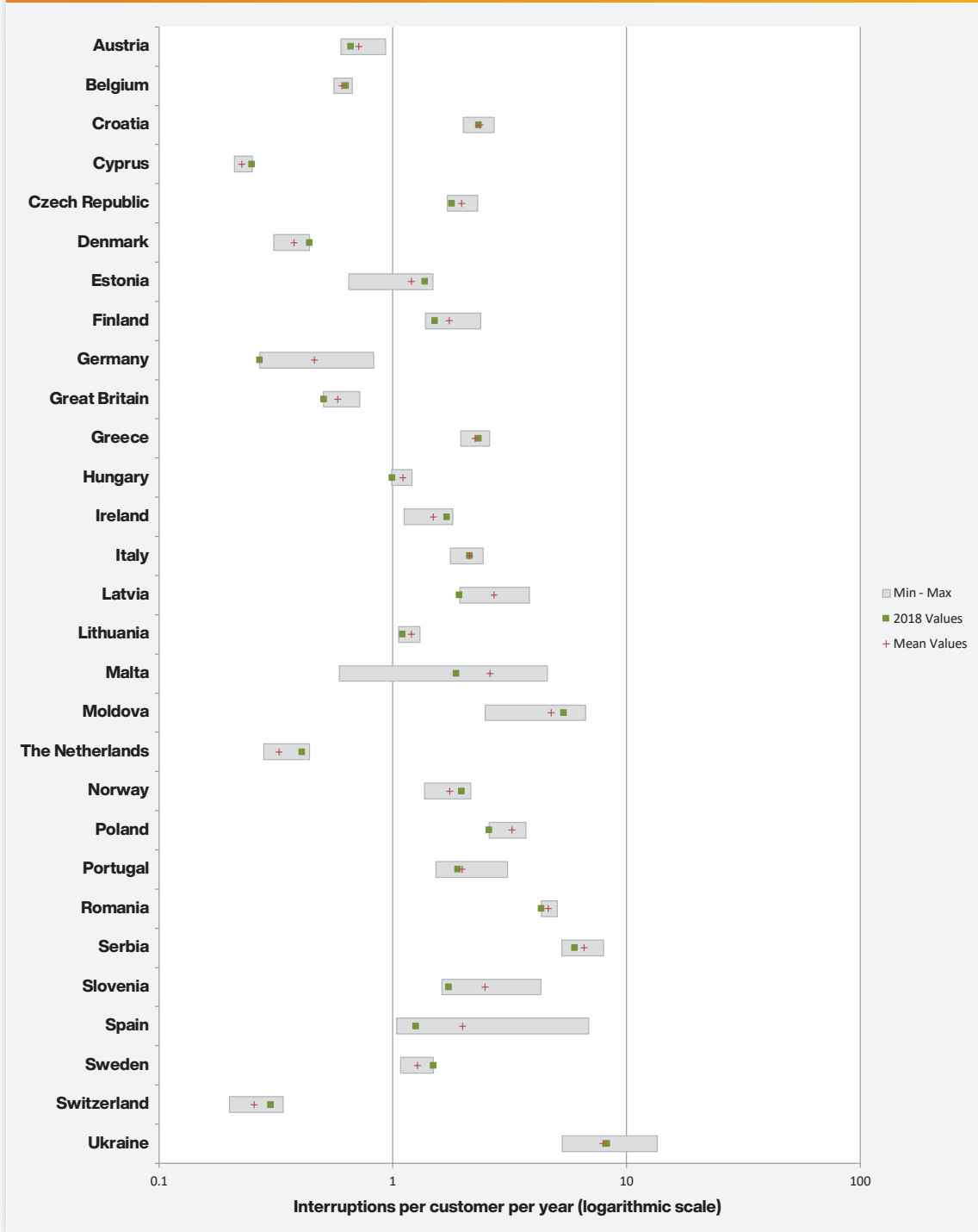
FIGURE 2-16: Unplanned long interruptions, SAIFI, all events (interruptions per customer per year) – boxplot
